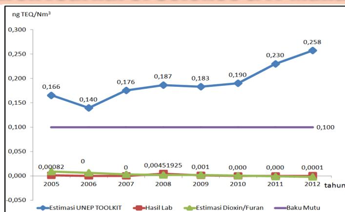
**Figure 9. Estimated Emissions of Dioxin/Furan at Cilacap Cement Plant by Multiple Regression Model**
