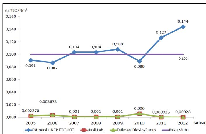
Figure 8. Estimated Emissions of Dioxin/Furan at Cilacap Cement Plant by Multiple Regression Model
